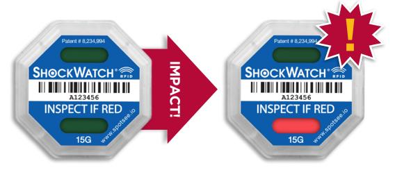
With stakes that significant, high-uptime web providers often affix multiple indicators per crate to capture impacts at multiple angles. If impacts occur, having multiple indicators provides overwhelming proof of impacts at specific, selected thresholds that range from 5Gs to 75Gs.
