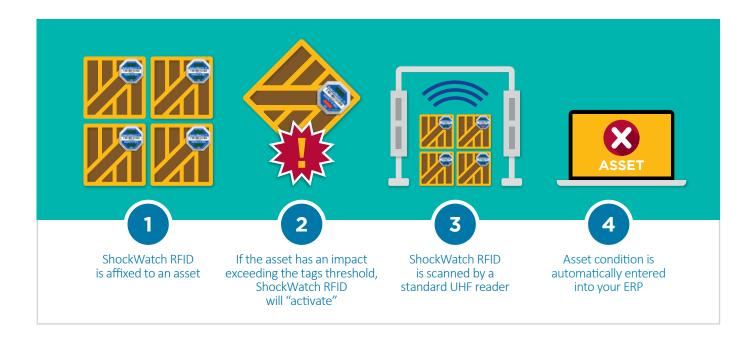
As passive RFID grows increasingly common, the benefits will increase. Passive RFID tags like SpotSee®'s are automatically read and recorded whenever a tag passes an RFID reader. Therefore, readers should be installed at choke points during shipping – like loading docks or transfer centers.
