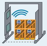
• As the damaged product is loaded on to the truck and passes by the RFID readers at the dock doors, the "impact event" associated with the specific product is automatically entered into the company's warehouse management system.
