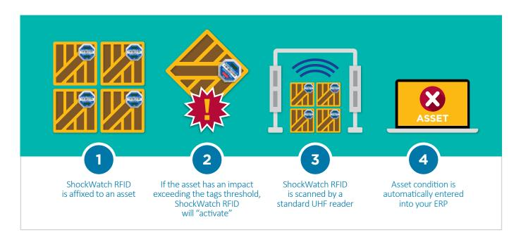
SpotSee's combination of impact monitoring and RFID is a bonus for manufacturers. Not only can cargo handlers and warehouse workers see at a glance which semiconductors or fabrication equipment has experienced potentially damaging impacts exceeding prespecified thresholds (between 5Gs and 75Gs), but that information can be automatically entered to inventory management systems whenever the tags near a passive RFID reader.
